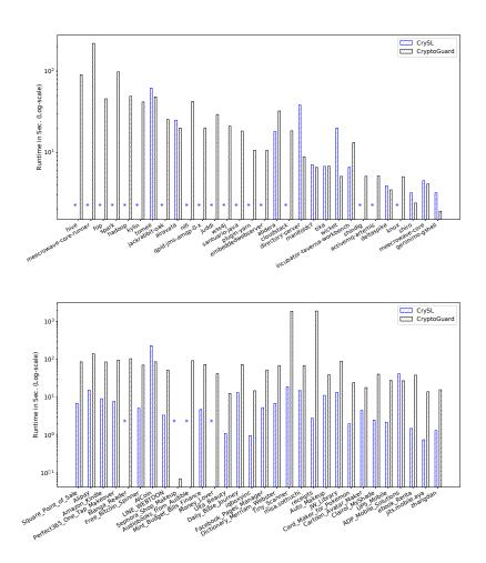
Figure 10: Runtime comparison in log scale of CryptoGuard and CrySL on 30 Apache root-subprojects in (a) and 30 Android applications in (b), ordered by decreasing lines of code (LoC). \* indicates crash. CryptoGuard successfully completed all tasks. The LoCs are shown in Table 8.
