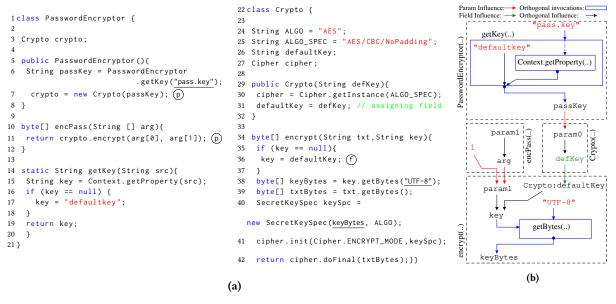
Figure 1: (a) An example demonstrating various features of CRYPTOGUARD. Crypto class is used for generic AES encryption and PasswordEncryptor class uses Crypto for password encryption. (f) indicates influence through the fields and (p) indicates influence through the method parameters. (b) Partial data dependency graph for keyBytes variable.
